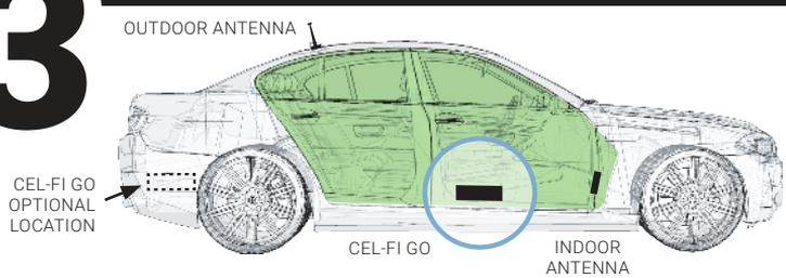
Find a good mounting location in your vehicle. Location should have some airflow, and be safe from bumps and external objects.
