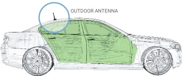
Mount your **Outdoor Antenna** on the exterior of the vehicle, towards the rear, according to its design, and the type of vehicle it's being used with. Make sure you consider the cable connection to the **CEL-FI GO** unit with your location choice.
